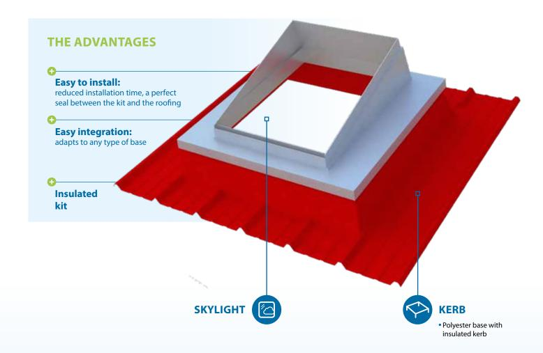
**The SKYDÔME® skylight integration kit (IFDT)** is designed to be fitted with a skylight (central rotation only) to adapt it to a sheeted roof or sandwich panel. This kit is composed of a polyester base with insulated kerb for optimum integration of a skylight, providing a discreet, aesthetic appearance.
